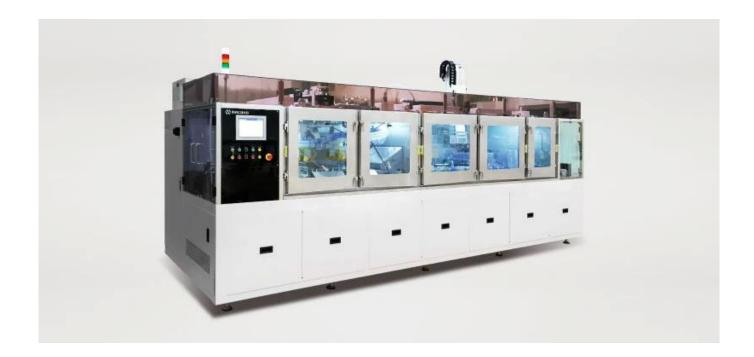
Full automatic processing from blasting to cleaning and drying can be done with one unit.
