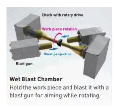
It is a semi-automatic device that handles super-hard blades one by one, and has provided more than 120 units to the world's largest manufacturers.
