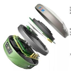
5. Built-in transceiver station: Adjustable from 0.5 to 2W, Supports a variety of transmission protocols, The operating distance is up to 5 km.
