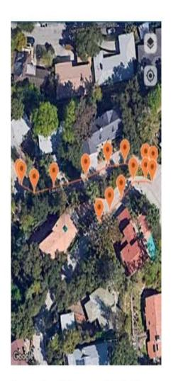
Create detailed maps of buried utilities in real time. Survey measurement data is added to GPS information to map the route of the tracked utility.
