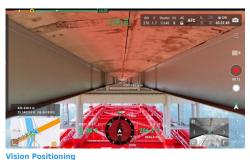
When GNSS is week or lost, the vision system can improve aircraft stability, for scenarios like bridge inspection
