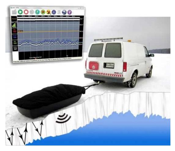
of <u>Underground radar</u> The IceMap $^{\text{m}}$  Real-Time Display displays the automatically detected bottom of ice (blue lines) in real time. Users can set a minimum thickness warning threshold (gold wire).
