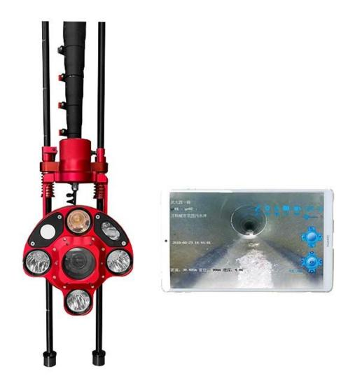
The GO1-H5 Integrated Pipeline Periscope System consists of hardware equipment and PipeX1H Pipeline HD Periscope Data Collection Software. During the discovery process, you can record and store internal images of detected objects in real time.
