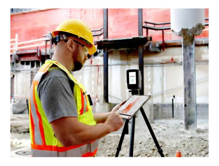
☑Scan distances of up to 350 m, expanding the scan range for each scan location
