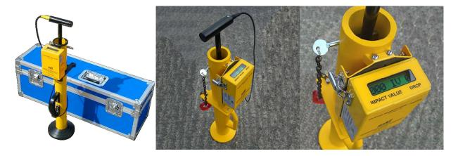
The 4.5 Kg CIST / 883 Clegg is produced by SDI (SD Instrumentation) and provides a simple and straightforward method of measuring and controlling soil strength and consolidation levels during the ditch recovery.883 The reading screen is clamped to the catheter and can be seen at the top during use.Single push-button program operation design, quite easy to use.
