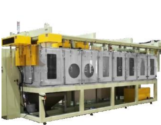
ILB-504 Automatic equipment capable of full- surface processing of complex shaped parts hung on a hanger
