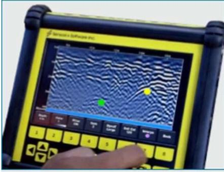
Handheld GPR device screen showing a radar scan with a green and yellow dot.
