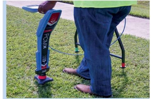
One second mapping measurements combined with simultaneous ACCA and ACVG data gathering makes surveying faster.
